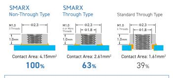
The world's first non-through type can secure a wider grounding area than that of the through type, which increases the substrate peeling strength and may reduce the return loss at high frequency. In a grounding connection, the non-through type is expected to increase or stabilize the shielding effect.
